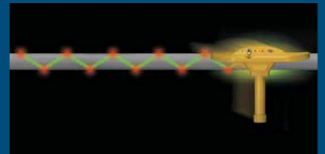
With the AML parallel with the pipe or underground object, you can now scan the entire length of the object's edge. As an alternative, utilize the "W" method of scanning by sweeping the area in a back-and-forth "W" motion, marking the object's location and run direction as it is tracked.
