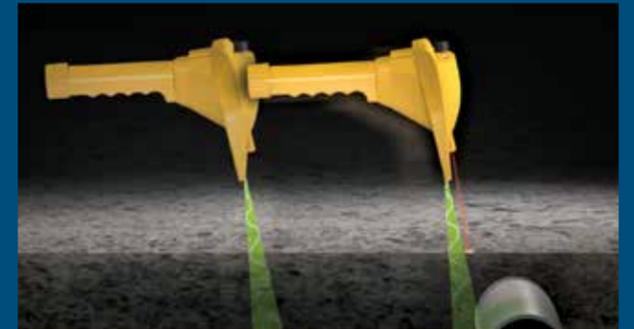
Holding the AML's handle parallel to the ground, scan the area of the undetectable buried object until one or both of the target indicators activate.
