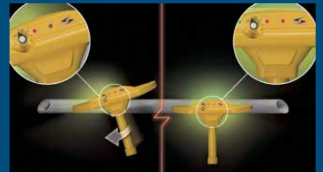
While the left or right target indicator is activated, rotate the AML until both LED target indicators light simultaneously, triggering the AML's tone and laser marker. This alert indicates that the pipe or object has been detected and that the AML is now parallel with the underground object.
